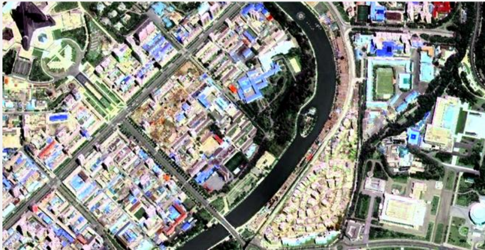
Figure 5. A pseudo-color composite image of the B2, B3 and B11 bands as the result of remote sensing image fusion by the proposed method.
