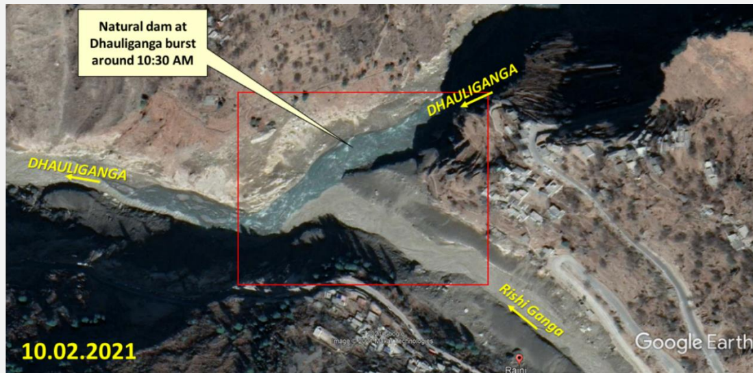
Figure 9. Google Earth image of 10 February 2021 brings a remnant of the broken natural dam, which can be realised clearly across the Dhauliganga River. As can be seen that heavy and abrupt moraine sediments (initially Rishiganga brought dark grey sediments as can be seen on both banks of Rishiganga River, and later it brought light grey sediments) were brought by the Rishiganga which initially blocked the flow of Dhauliganga. However, due to heavy flow in the Rishiganga, the temporary natural dam could not sustain and broke quickly, causing a devastating flash flood in the downstream stretch of Rishiganga
